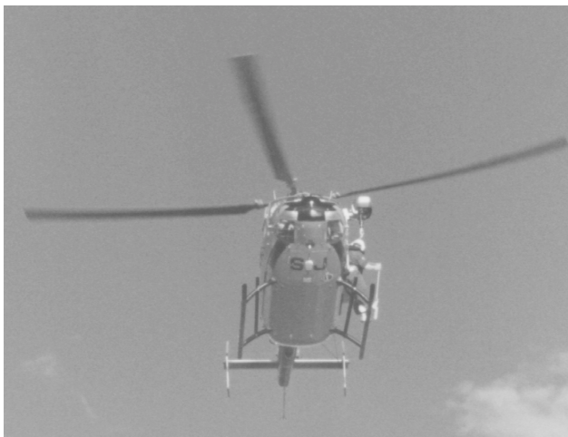
Figure 1. The NEST helicopter approaching the dive boat with the winchman standing on the skid holding the weighted Hi-line.
