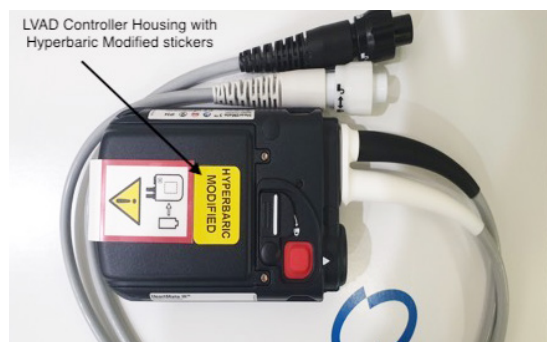
Figure 2 Hyperbaric modified LVAD controller
