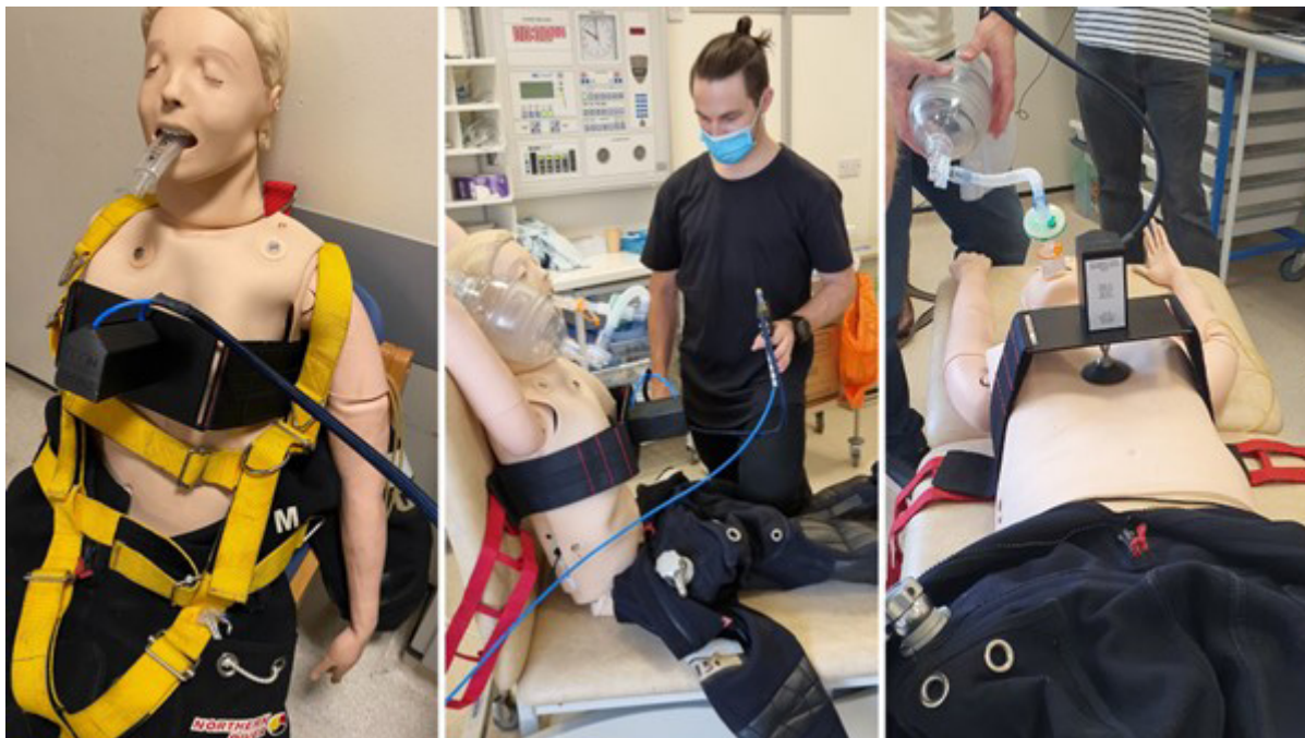
Figure 2 The NUI Compact Chest Compression Device (NCCD) in use on a manikin
