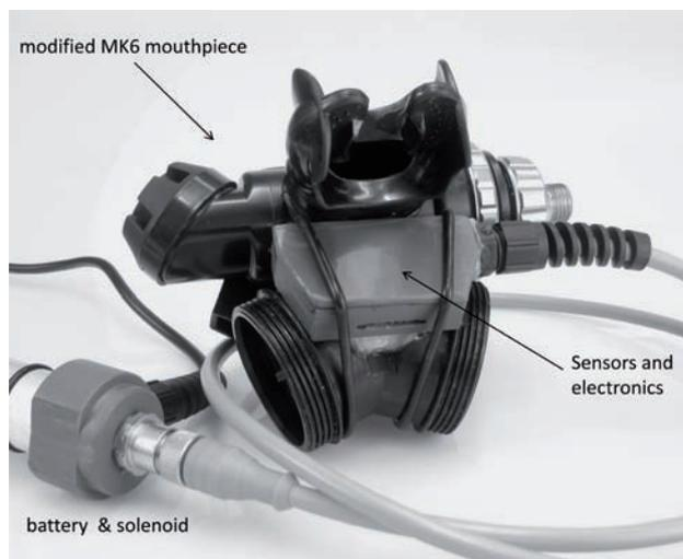
In a final study to measure breath-by-breath PO<sub>2</sub> and PCO<sub>2</sub>, a subject (35-year-old male) breathed through the rebreather mouthpiece. In all studies, repeat observations were made. The CO<sub>2</sub> transducer was two-point calibrated with air (assuming 350 ppm CO<sub>2</sub>) and with air containing 1% CO<sub>2</sub>.
