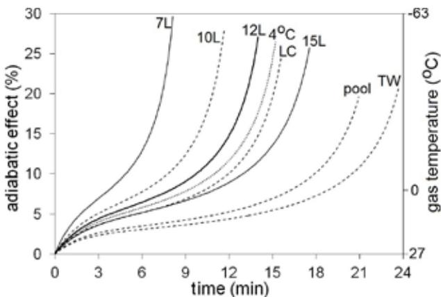
water, high gas consumptions give a similar effect as with an ordinary dive (20 msw, 25 aL·min<sup>-1</sup>) in temperate water (compare 'pool' and 'TW' curves).
