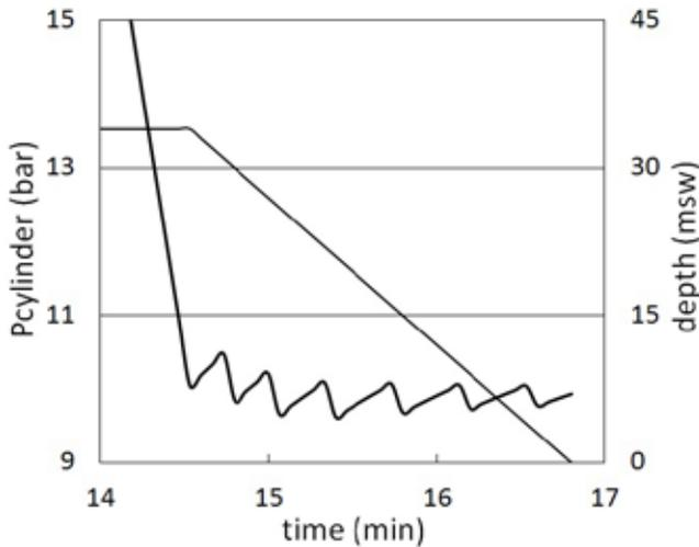
$A_{effect}$  diminishes, unless the cylinder pressure approaches 10 bar, then,  $A_{fraction}$  (Figure 4) rises.  $AP_{effect}$  shows a flat maximum somewhere near the middle of the dive.
