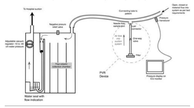
and if the rate of pressurisation was limited to 10 kPa·min<sup>-1</sup> or less. Under these conditions the water-seal was maintained and the column of water making the seal did not back flow into the collection chamber.<sup>5</sup>
